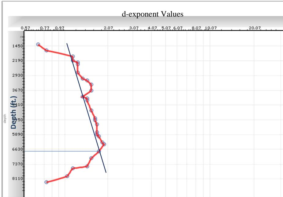
**Figure (2) Modified d-exponent method to determine abnormal pressure depth in well (A1).**
