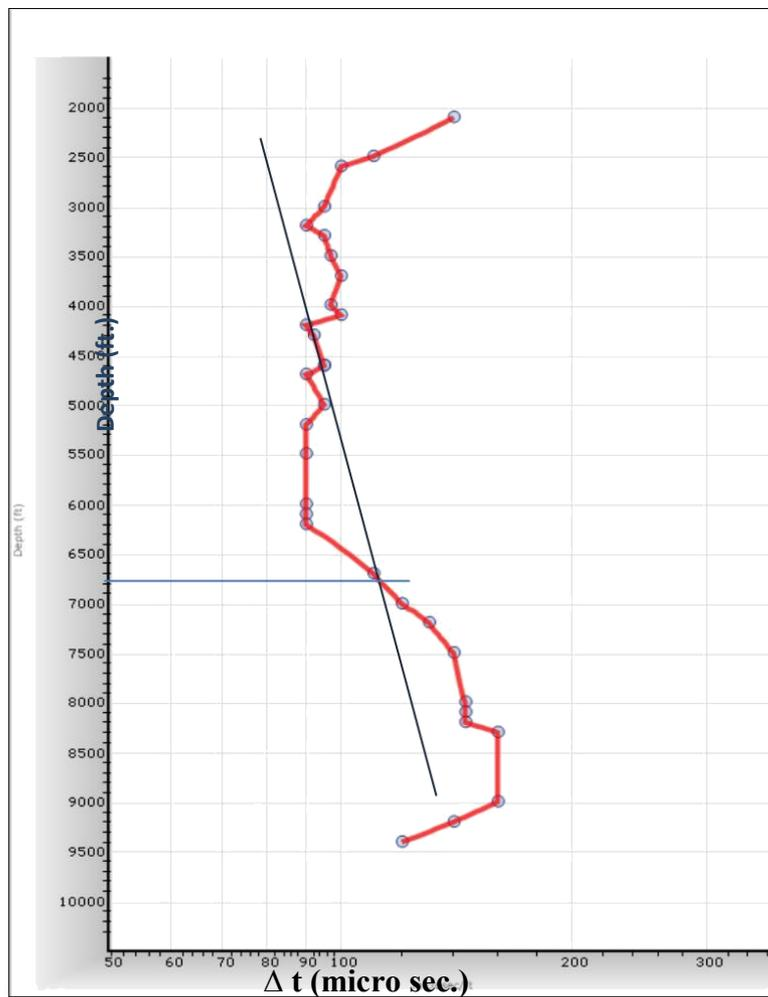
**Figure (4) Prediction of abnormal pressure depth using transit time ( $\Delta t$ ) in well A1.**
