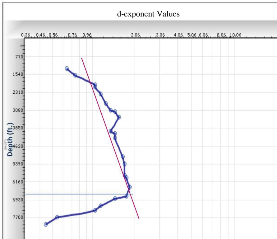
**Figure (3) Modified d-exponent method to determine abnormal pressure depth in well (A2).**
